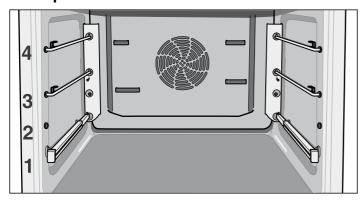
The cooking compartment has four shelf positions. The shelf positions are counted from the bottom up.
