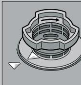
screw on filter system. NOTE MARK!
