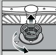
Rotate filter cylinder, remove filter system ...
