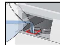
**i** If the water tank filter is dirty → clean the filter in the water tank. See page 4.
