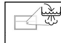
2. Remove the condensate tank completely.
