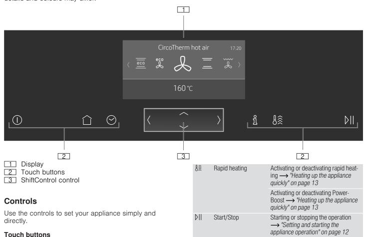
There are sensors under the touch buttons. Touch on the corresponding touch button to select a function.
