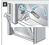
Left lock: Anti-clockwise Right lock: Clockwise
