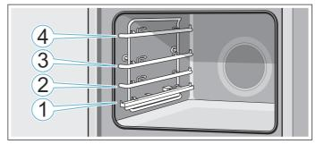
The accessories can be pulled out approximately halfway without tipping. You can use the pull-out rails to pull the accessories out further.
