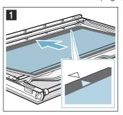
Push the intermediate panel downwards in the a area, insert the b holder at an angle and push down until it locks into place (Fig. 2).
