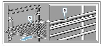
When inserting baking trays, ensure that the catch tappet **a** is at the rear and is facing downwards. The sloping edge of the accessory **b** must be facing forwards towards the appliance door.
