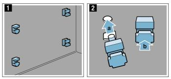
3. Use the hook to attach the rear holder into the upper hole **a** and push it into the lower hole **b** (fig. **3**).
