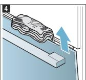
6. Push both retainers at the top of the intermediate panel upwards, but do not remove them (fig. 5). Hold the panel with one hand. Take out the panel.
