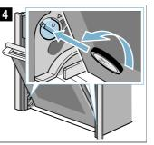
Left-hand lock: Anti-clockwise Right-hand lock: Clockwise
