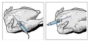
**Turning the food:** If you wish to turn the food, do not remove the meat probe. Once you have turned the food, check that the meat probe is correctly positioned in the food.
