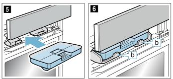
Slowly push the control panel downwards and then towards the rear until it is closed completely. The water tank has been filled. You can start operations with steam.
