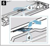
10. Lift the first and second intermediate panels from below (fig. 2) and remove them in the direction of the arrow (fig. 3).
