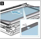
5. Push down on the intermediate panel around b, slide the holder c in at an angle and push down until it clicks into place (Fig. 6). The holder has been inserted (Fig. 7).
