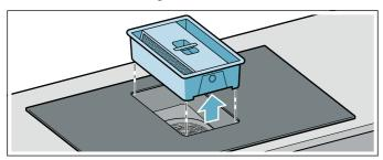
**3.** Press down on the two catches on either side of the container to separate the metal grease filter from the container.
