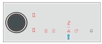
3. To set a different fan setting, touch the \$\mathcal{L}\$ symbol and use the twist knob to select the required setting. The fan setting that is selected will be shown on the display panel.
