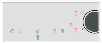
**2.** Within the next 5 seconds, select the required temperature setting using the twist knob.
