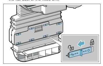
2. Open the drawer in the flat duct and remove the activated charcoal filter.
