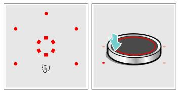
Position the twist knob on the twist pad so that it is in the centre of the indicators which delimit the twist pad area.
