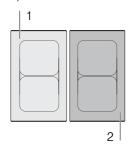
**Note:** In the combi zone, the PowerBoost function can only be activated if the two hotplates are used independently of each other.
