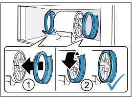
2. Slide the odour filter into the filter retainer.
