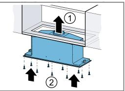
2. Tighten the fastening screws.
