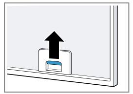
**3.** Remove the grease filters from the holders. To prevent grease from dripping, hold the grease filter horizontally.
