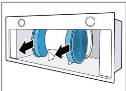
**3.** Guide the odour filter around the motor.
