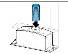
Establish the connection to the exhaust air opening.
