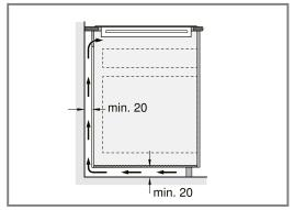
**2.** Ensure that an opening at the top of the rear of the unit is unobstructed.
