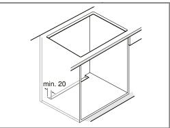
**4.** Do not hermetically seal the lower base. **Note:** If the appliance is installed in an island unit or in another location that is not described here, guarantee that the hob is ventilated appropriately.
