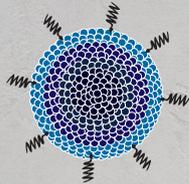
Microwaves are able to penetrate food items to a depth of 1 cm. This causes the water, fat and sugar molecules in the food to vibrate causing friction which in turn causes heat.
