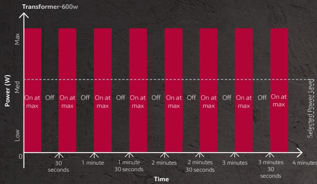
Traditional microwave replicate lower power levels by delivering power at maximum or completely off
