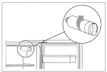
**4.** Screw in the water filter in clockwise direction and make sure it is firmly fitted to the water filter base.
