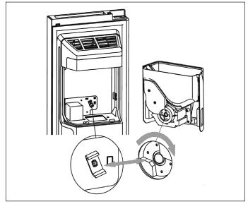
1. Check that the two couplers are at a suitable angle to connect correctly. If necessary, turn the coupler of the ice bucket to match the motor coupler.
