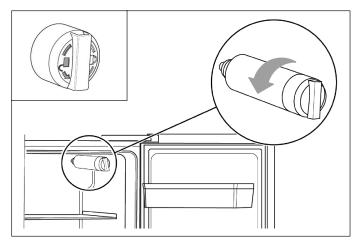
Screw out the old water filter in anticlockwise direction (see sign on the filter) and remove it.
