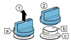
To put the control knob back on, press it on at its original position.
