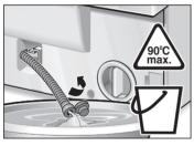
☐ Push up the closing cap (1st) and place the drain hose back in its holder (2nd).
