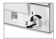
☐ Carefully remove the pump cap.
