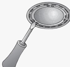
3. Replace the halogen light bulb (conventional halogen bulb, 12 Volt, max. 20 Watt, G4 cap).
