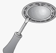
3. Sostituire la lampadina alogena (lampadina alogena commerciale, 12 Volt, max. 20 Watt, attacco G4).
