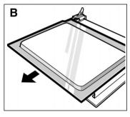
3. Raise the upper panel and remove it. (Fig. B)
