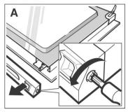
The glass panel on the oven door can be removed to assist in cleaning.
