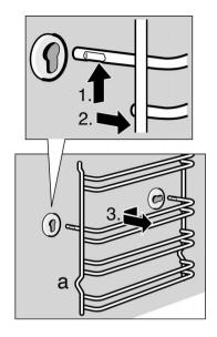
The rails can be removed for cleaning.
