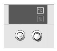
A default value appears if you have selected a type of heating using the function selector. Set the temperature or cleaning level required using the temperature selector.
