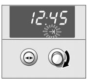
6. Extend the end time using the rotary knob.
