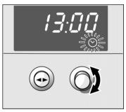
2. Use the rotary knob to set the time while the ⊗ symbol is flashing.
