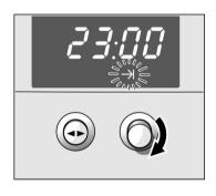
4. Extend the end time using the rotary knob.
