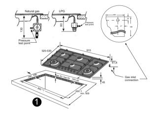
Before connecting the unit, check whether the local connection conditions (type of gas) are compatible with the unit's setting. Observe any special conditions imposed by local suppliers (utilities). The specifications of this cooktop are stated on the data label located on the bottom of the cooktop base.
