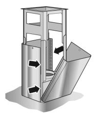
**4.** Push up the upper flue part and secure with 2 screws.
