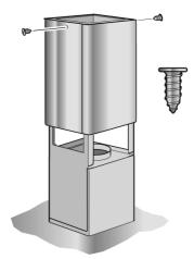
**5.** Insert the two lower parts of the flue and push together.
