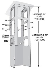
**NOTE:** The support frame can be aligned subsequently by loosening the fastening screws on the ceiling.
