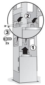
**3.** Hook in retaining clip and screw tight.
