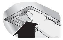
2. Replace the defective bulb with a new one of the same type and equivalent power (see rating plate).
