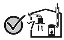
Adequate intake air must therefore always be provided.
