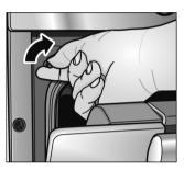
Turn the door contact switch clockwise. The NeffLight® is switched off.
