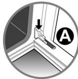
To re-fit the door, carry out the instructions given above in the inverse direction. When the hinges **B** are back in their seats, open the door all the way and re-fit the safety catches of the hinges, lowering the respective pins **A** (one for each hinge).
