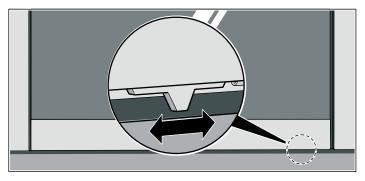
To switch off the NeffLight®: Slide the door contact switch to the right.
