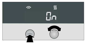
After reaching the set temperature, Rapid heat up switches off. The  $\mbox{\tt II}$  symbol goes out.
