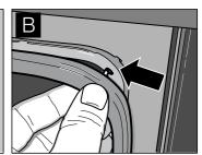
Check again to ensure that the seal is seated correctly in the corners in particular.
