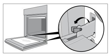
The hinges are secured and cannot snap closed.
