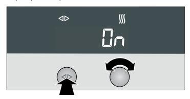
After reaching the set temperature, Rapid heat up switches off. The  $\ensuremath{\mathbb{M}}$  symbol goes out.
