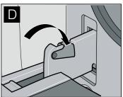
The appliance door is secured and can no longer be removed.
