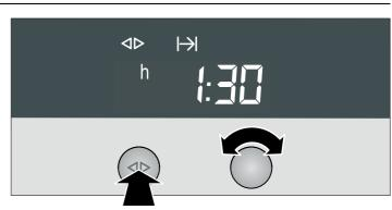
Once the cooking time has elapsed, the appliance switches off automatically.
