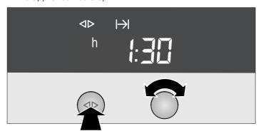
**5.** Turn operating mode selector to oposition and press in. Once operation time has elapsed, the appliance switches off automatically.
