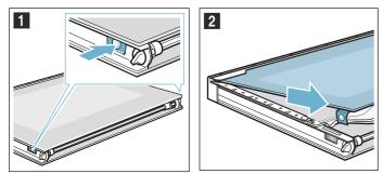
Push the intermediate panel downwards in the a area, carefully lift the b holder until it can be pulled out (Fig. 3).
