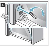
Left lock: Anti-clockwise Right lock: Clockwise
