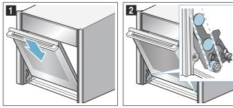
Turn the door handle upwards slightly a so that the appliance door slides downwards fully b (Fig. 3).
