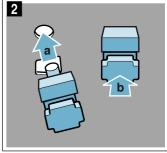
3. Use the hook to attach the rear holder into the upper hole **a** and push it into the lower hole **b** (fig. **3**).
