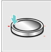
Position the twist knob on the twist pad so that it is in the centre of the indicators which delimit the twist pad area.
