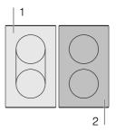
**Note:** In the combi zone, the PowerBoost function can only be activated if the two hotplates are used independently of each other.
