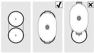
When you are using cookware on just one of the two hotplates, it can be moved to the second hotplate. In this case, the heat setting and the selected settings are transferred.
