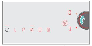
The function has now been activated. The 😹 temperature symbol flashes until the frying temperature is reached. A signal sounds and the temperature symbol lights up.
