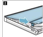
Push down on the intermediate panel around a, carefully lift the holder b until it can be pulled out (Fig. 3).
