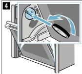
Left-hand lock: Anti-clockwise Right-hand lock: Clockwise
