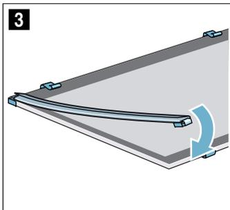
3. Insert the intermediate panel with the seals and spacers. The arrow on the intermediate panel must line up with the arrow on the frame (Fig. **4**).
