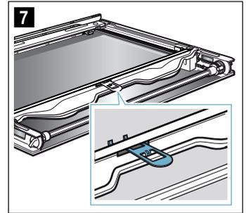
6. Insert the inner glass into the mounting rail **d** at an angle towards the back (Fig. **8**).
