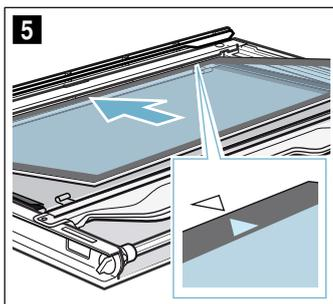
5. Push down on the intermediate panel around **b**, slide the holder **c** in at an angle and push down until it clicks into place (Fig. **6**).
