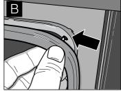
**2.** Hook the door seal in at five further points (Fig. C) by turning the hooks slightly (Fig. D).
