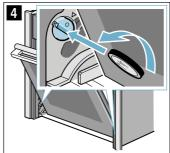
Left-hand lock: Anti-clockwise Right-hand lock: Clockwise
