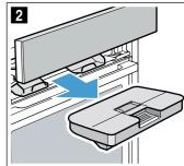
4. Press down on the cover along the seal to prevent water from leaking out of the water tank.
