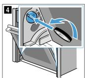
Left-hand lock: Anti-clockwise Right-hand lock: Clockwise
