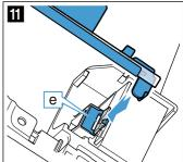
**10.** Insert the second reflector on the right-hand side in the same way as the left-hand reflector.
