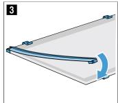
3. Insert the intermediate panel with the seals and spacers. The arrow on the intermediate panel must line up with the arrow on the frame (Fig. 4).
