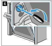
Left-hand lock: Anti-clockwise Right-hand lock: Clockwise
