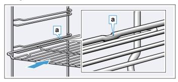
When inserting baking trays, ensure that lug  $\mathbf{a}$  is at the rear and is facing downwards. The sloping edge of the accessory  $\mathbf{b}$  must be facing towards the appliance door.
