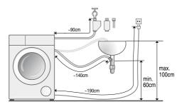
**Note:** If the hose holders are used, the possible hose lengths are reduced!
