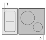
**Note:** The PowerBoost function can also be activated in the flexible area if the cooking zone is being used as a single hotplate.
