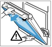
**Note:** If you are unable to release the front panel, use one hand to take hold of the top edge of the front panel and pull it in the direction of the arrow until it is released.
