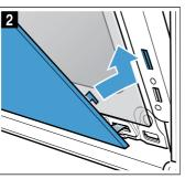
**Tip:** If you are unable to click the front panel into place, check whether the front panel is touching the handle. Open the door a little further until the front panel clicks into place.
