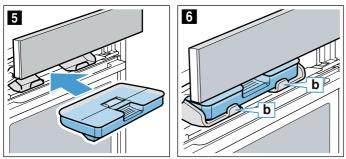
**9.** Slowly slide the control panel downwards and then push it towards the rear until it is closed completely. The water tank has been filled. You can start using operating modes with steam.
