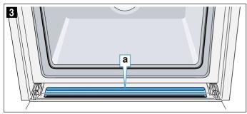
**Note:** If the seal has become detached, fit the seal back onto the drip trough.  $\rightarrow$  "Appliance door" on page 36
