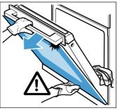
**Note:** If you are unable to release the front panel, use one hand to take hold of the top edge of the front panel and pull it in the direction of the arrow until it is released.
