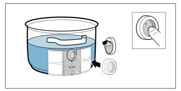
**3.** Press down all over the surface of the silicone patch, including in the centre.
