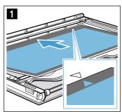
Push the intermediate panel downwards in the a area, insert the b holder at an angle and push down until it locks into place (Fig. 2).
