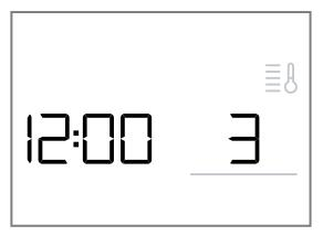
After operation starts, the thermometer lights up and the bars next to it light up one after another to display the heating up progress of the interior temperature. When all the bars are lit, the appliance has reached the set temperature. When using the grill, all the bars are lit from the start.
