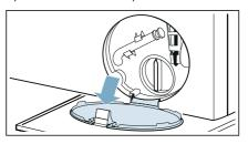
**3.** Take the drain hose out of the retainer.
