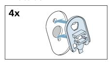
4. Lock the covers firmly in place by applying pressure to the snap-in hooks.
