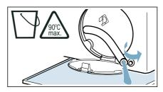
4. Carefully unscrew the pump cover; residual water may leak out. Clean the interior, pump cover thread and pump housing. The impeller in the drain pump must be able to rotate.
