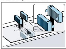
6. Insert the grease filter.
