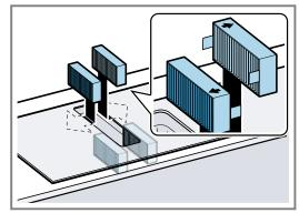
6. Insert the grease filter.
