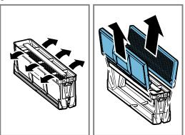
**2.** Place the individual components of the grease filter loosely in the dishwasher and do not jam them in.
