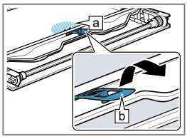
5. Lift the first and second intermediate panes from below 1 and remove them in the direction of the arrow
