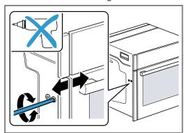
Turning the screws clockwise makes the gap larger Turning the screws anti-clockwise makes the gap smaller
