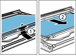
6. Remove the spacers a and seals for cleaning, if required.
