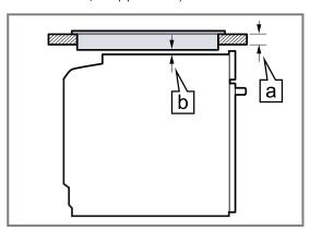
The minimum worktop thickness b is based on the required minimum clearance a.
