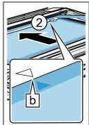
The arrow on the intermediate pane must line up with the arrow on the frame b.
