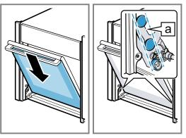
2. Ensure that the appliance door slides the short distance remaining to the bottom.
