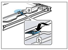
The retainer has been inserted.
