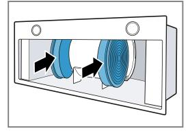
4. Install the grease filters.
