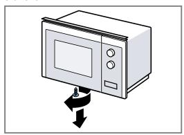
2. Remove the cover at the base of the microwave.
